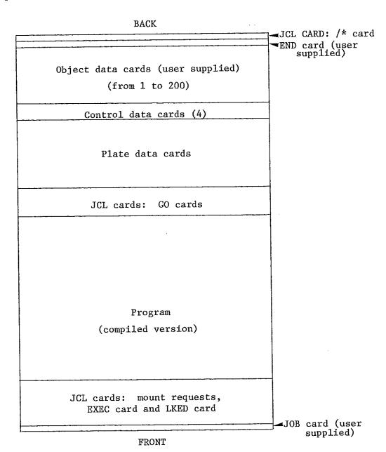
(One exception to this deck setup can arise because of plotting. In generating a plot, the IBM 360/40 writes the plotter commands onto a user supplied magnetic tape. This tape is read by the PDP-11 which controls the plotting. We have been using SCØ357 as a scratch tape for this purpose and other users are free to do the same, or they can supply their own scratch tape. The current general use scratch tape will be listed on the program box.
