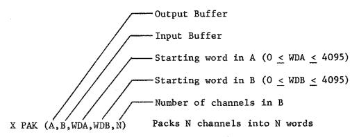
Each channel in B consists of 2 12-bit words. Starting at WDB in buffer B and processing N such channels, the low order word of each channel is stored into consecutive words in buffer A, starting at WDA. The high order words of each channel in B are ignored.
