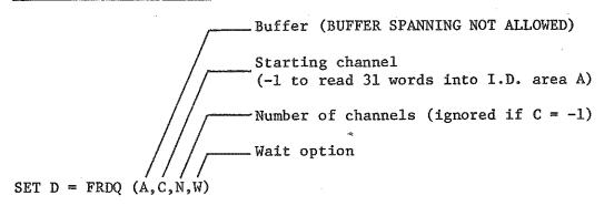
Starts reading N channels from IBM tape to buffer A. Reads to end of buffer if N = 0. Works like READ command except:
