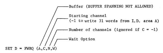
Starts writing N channels to IBM tape from buffer A, starting in channel C. Writes to end of buffer if N=0. Works like WRIT command except for the same 4 differences described under the RDQ command above. Also, if a WRQ command is directed to a write protected IBM tape, a ?6273?00.00 error is given.
