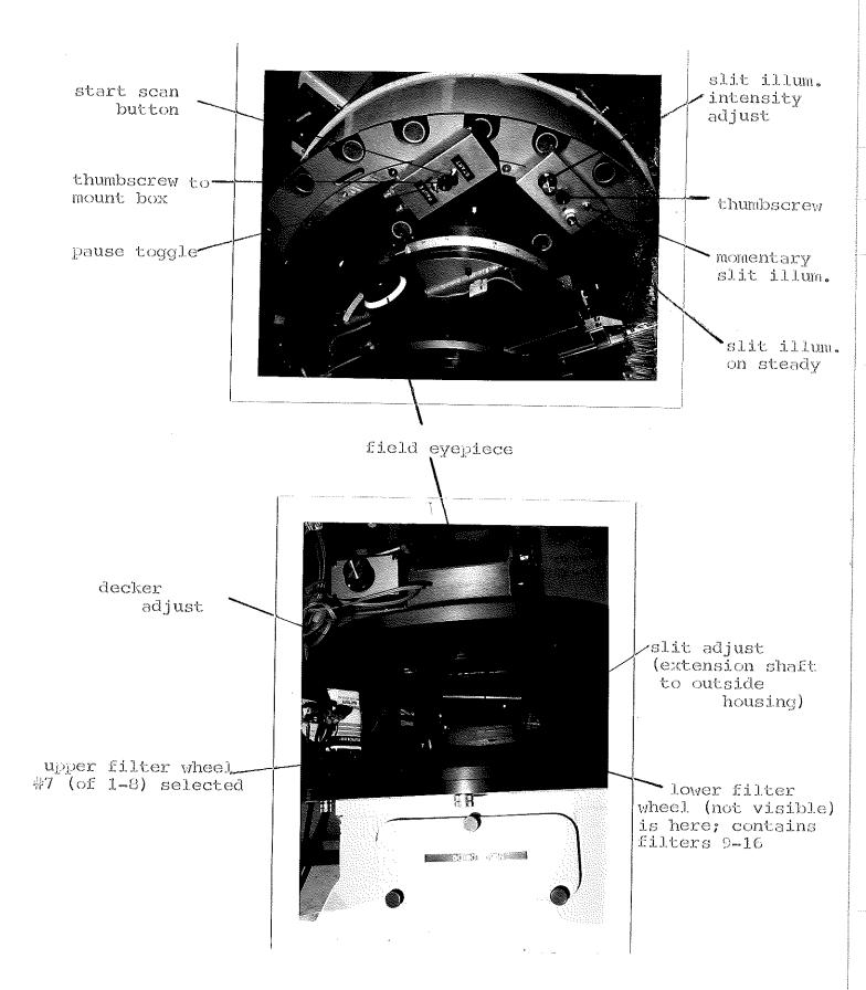
Note: Filter wheels inside access door are 1" square or round and may be added/changed with difficulty and prior notice. The 2" square filter holder is higher in the beam and easily accessible to users.
