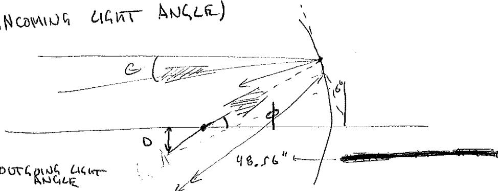
$\phi = 12^\circ - \theta = 11.44^\circ$  - OUTGOING LIGHT ANGLE
